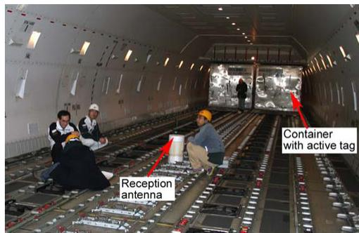
**Fig. 1 – Configuration of Emission Measurement in Boeing 747-400 Freighter**
