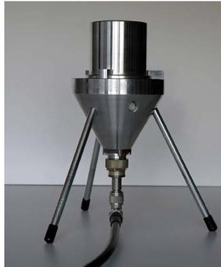
Fig. 1 – Open-Ended Coaxial Line Probe
