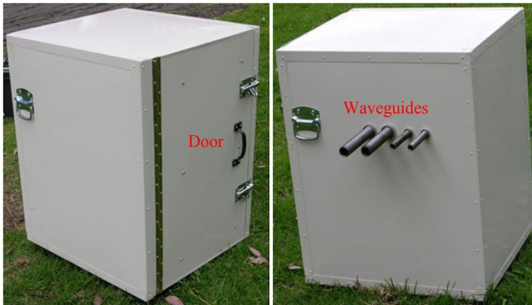
Fig. 1 – Shielded Cabinet. Note the door and the waveguides for input signals
