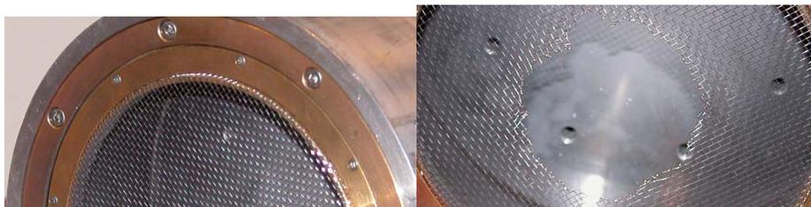
Fig. 1 – Example of wear in a stainless steel anode mesh.
