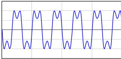
Fig. 3 The form of a signal when  $\Delta R \gg \lambda_0$
