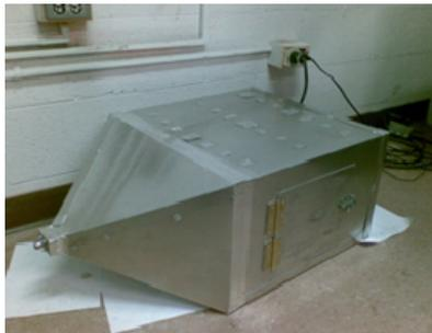
Fig. 1 – TEM cell used in this study
