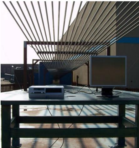
Fig. 1 – NEMP Testing of PCs setup
