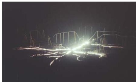
Fig. 2 – The fragment of spark channel luminescence in the neighbourhood of the grounding rod
