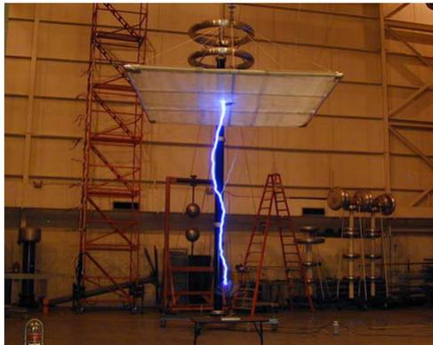
Fig.1 Breakdown on the spline ball ionizer
