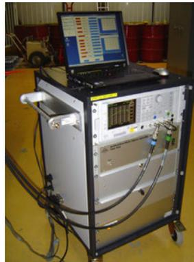
Fig. 1 – BCI Test bench for complex cables
