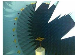
Fig. 3 – Antenna Measurement Setup
