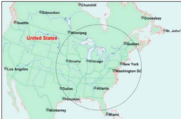
Fig. 1 – Area covered by the early-time HEMP from a 170-km burst over the United States
