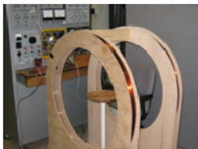
Fig 1 – Helmholtz coil used for magnetic field analysis
