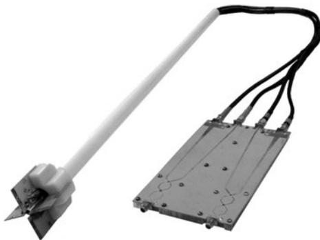
Fig. 1 - Active receiving antenna with dual polarization
